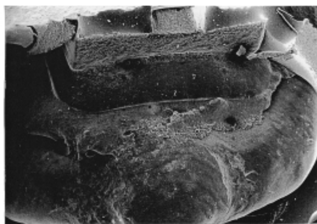
FIG. 3 (a) SEM photo of enamel/composite/bracket interface of extracted tooth. (b) SEM photo of replica cast of same area of tooth as in Fig 3a. Score 2—good reproduction/fine detail visible.
